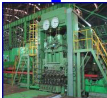
Hot Levelling Process
